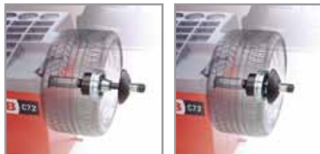
Pneumatic locking mechanism of the wheel.
