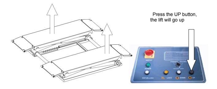
When the lift is working (lifting a car), remember:
